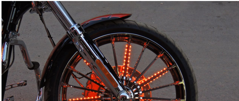
Example of “leading” and “Trailing” edge LED mounting on spokes.
