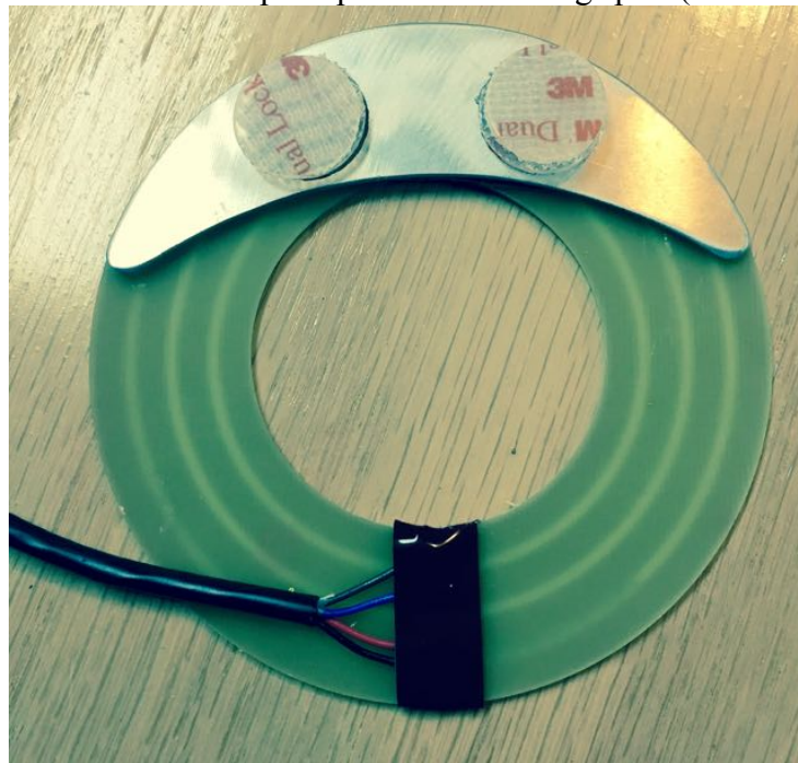
Splice Plate installed on back of PUC Ring. PUC Ring should be on bike before installing.
