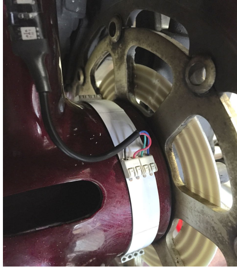
Note minimal wire between the LED and Backbone in the picture above.
