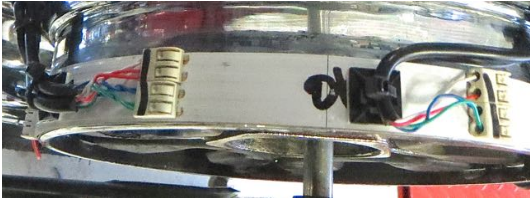
Example installation and use of wire ties and wire tie mounts.
